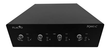
PQ Series portable dynamic signal conditioner is characterized by high sampling rate, high measurement accuracy, compact size and portability.  $24\,\Delta - \Sigma$  data acquisition chip, multichannel synchronization and sampling frequency up to  $88\,$  kHz/per channel. Customer can achieve the equipment control and data acquisition, signal analysis and other functions through supporting software SoundExpress.
