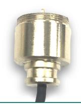
PNS20 preamplifier is a voltage powered preamplifier with high input impedance, low background noise and wide frequency response range. It can be used with MP21 1/2 inch prepolarized measurement microphone, and also compatible with other brands measurement microphones such as B&K, GRAS. The output adopts a three wire system plug, which can be easily configured for power supply and signal output. It is suitable for electroacoustic tester, multichannel analyzer and other instruments.
